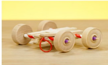
Prototype two mechanism: a rubber band is used to slingshot the car forwards.
