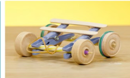
Prototype three mechanism: a rubber band is wound around the back axle and unwinds to make the car move.
